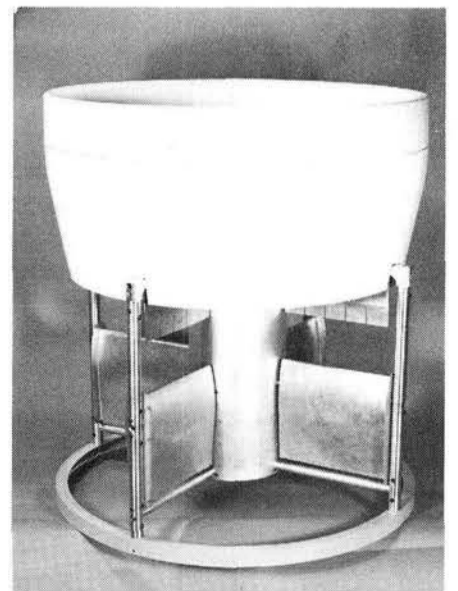
FULL-SCALE MODEL of the AROD (Airborne Remote Operated Device), a small, highly mobile aerial reconnaissance vehicle, is 30 inches in diameter at the top and 5 feet tall.
